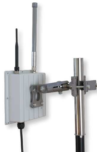
YellowJacket ZigBee Outdoor WiFi Hive Unit rear view shows Universal Mounting Bracket
